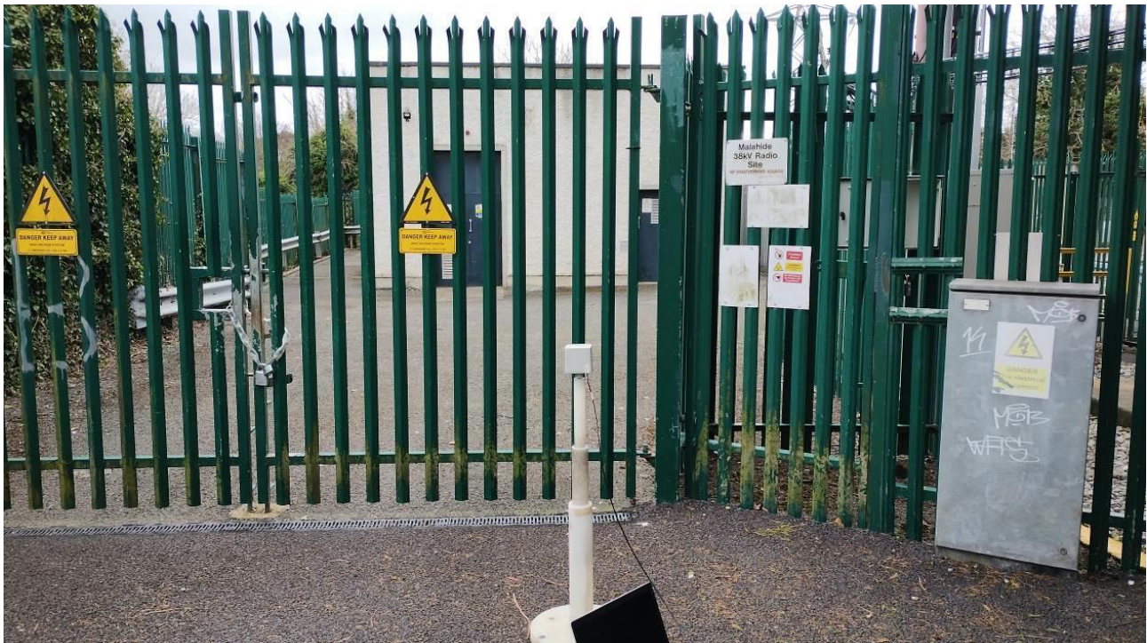
Image 22-73 EHP cube measuring AC fields.
