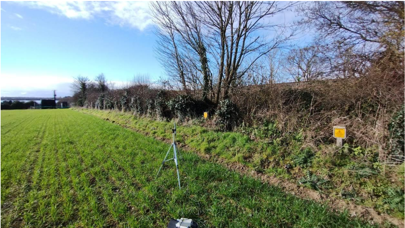
Image 22-53 Bartington magnetometer taking DC and near DC measurements at Donabate.
